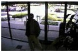
Typical image from CCD showing saturated highlight and unrecognizable dark.
