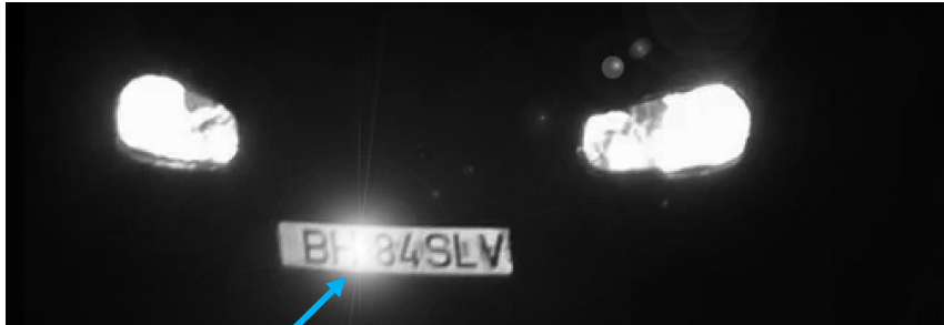
Ghost image on license plate (Typical lens)
